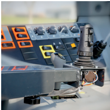
Comandi interno cabina con joystick Parker a 4 assi e centralina programmabile. Commands inside cabin with Joystick Parker 4-axis and programmable control unit.
