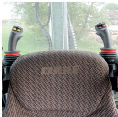
Comandi interno cabina con joystick Danfoss. Commands inside the cabin with joystick Danfoss.
