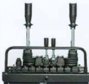
Posto guida a terra con distributore elettroidraulico. Driver's seat on the floor with electro-hydraulic distributor.
